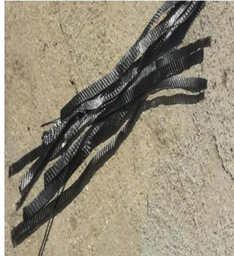
Figure 3. 20mm CFRP strips
