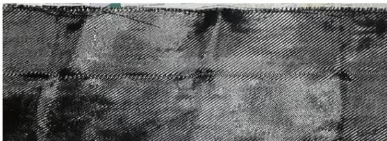
Figure 1.CFRP Fabric
