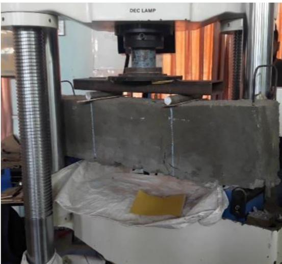
Figure 6. Two point load test setup
